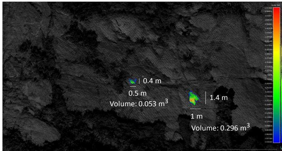
Figure 2: Two examples of cluster classified as rockfall coloured with the distance parameter calculated perpendicularly to the Montserrat cliff surface. Monitoring dates: Decembre 2017 - July 2018
