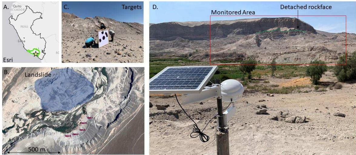
Figure 1: Site setup and location of monitored landslide. A. Location of landslide in Siguan Valley southern Peru (modified Graber et al. 2020; data Esri) B. Satellite image showing location of cameras and landslide being monitored (imagery CNET/Airbus). C. Installation of one of six coded targets on the landslide. D. Time-lapse photography setup and area of landslide being monitored.
