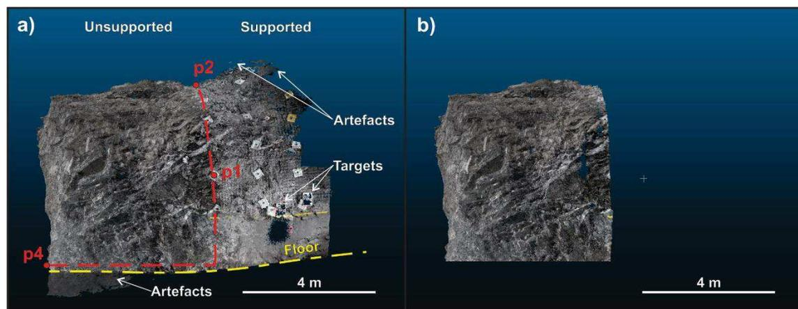
Figure 1: Sideview of a development face. a) Untrimmed mesh, which includes artefacts. The red dashed line delineates the region shown in (b). b) Trimming the data excludes the ground support mesh and the floor of the development.
