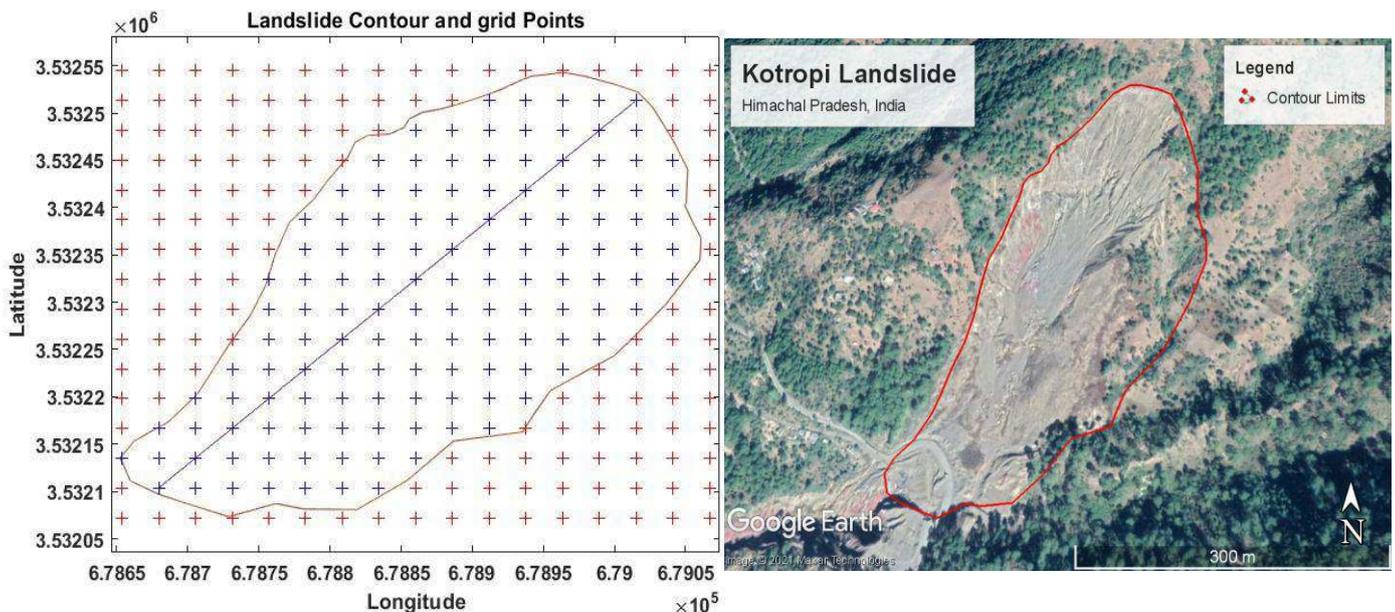
Figure 1: Location of the landslide(Right side) and the gride points and elevation line passing through the highest and lowest elevation points(Left side). The Z value for each point will be calculated using a spline curve.
