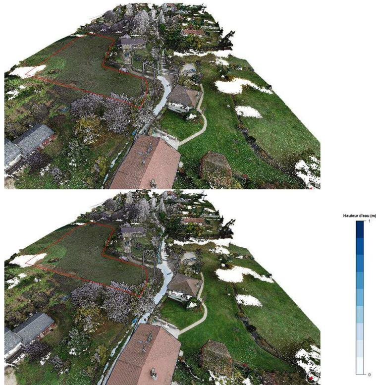
*Figure 2 Representation in 3D, with the Rim-Nat platform, of the flood wave with high resolution DEM. In red line, the study area limits. At the middle of the figure, white and blue areas are the water depth*
