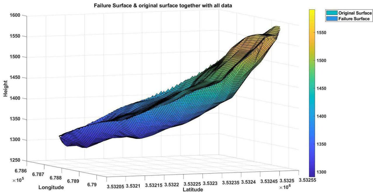
Figure 2. 3D-View Kotropi Landslide with Failure surface and original surface together. Posted after refining the gride
