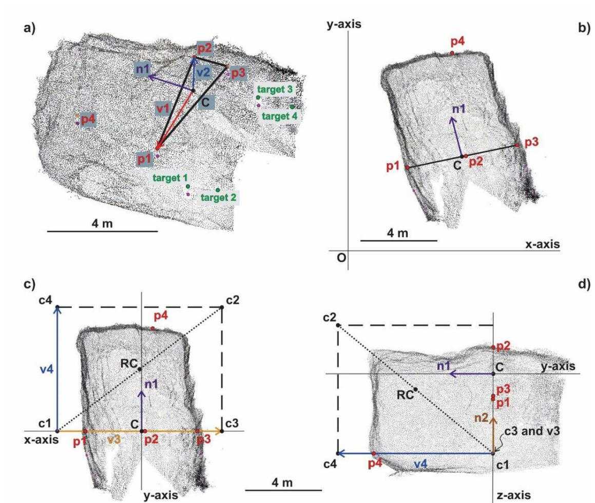
Figure 2: Steps involved in modifying the region of the capture. a) The centroid of triangle ( $p1 - p3$ ) forms the origin of a coordinate system translation ( $C$ ). c) Using geometry and a transformation matrix, the capture is translated and rotated, so that the normal ( $n1$ ) of triangle ( $p1 - p3$ ) is parallel to the  $y$ -axis and its direction used to determine which side of the  $x$ -axis to keep. d) The box defined by the dashed black line is the part of the capture that is kept.
