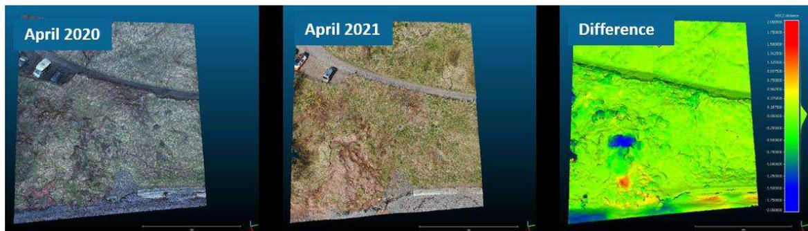
*Fig 2. Quantifying the magnitude of landslides in successive surveys from Catterline Bay*
