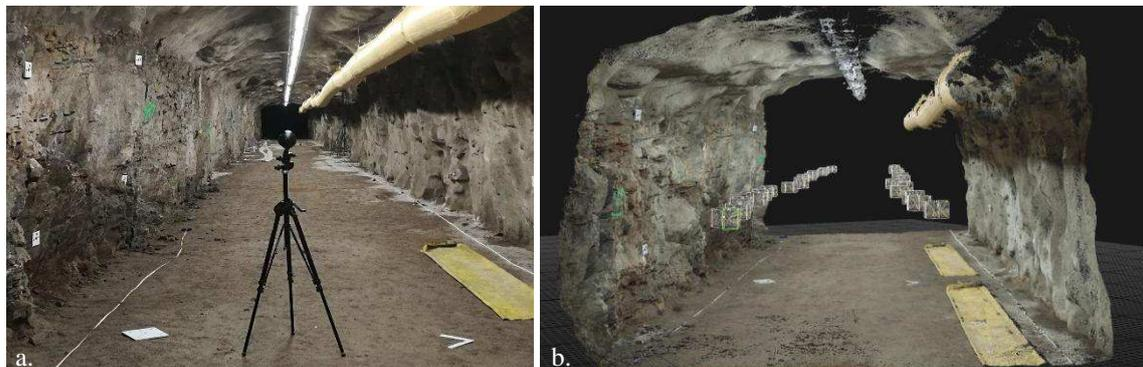
Figure 1: Image acquisition with the 360-degree camera at the test site of the Underground Research Laboratory of Aalto University (a), and the 3D model of the site reconstructed with SfM photogrammetry (b).
