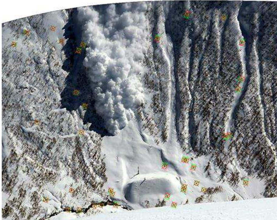
Figure 1: Oblique and unrectified image of the avalanche approaching the instrumented embankment dam; image used for mono-photogrammetric reconstruction and measurement of avalanche characteristics.
