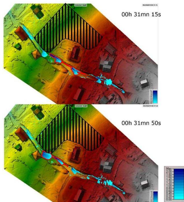
Figure 1 Result of the 2D non-permanent flow modelling with high-resolution DEM
