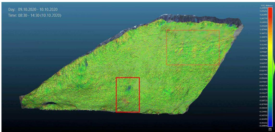
Figure 2: Landslide detection and quantification within the bank area.
