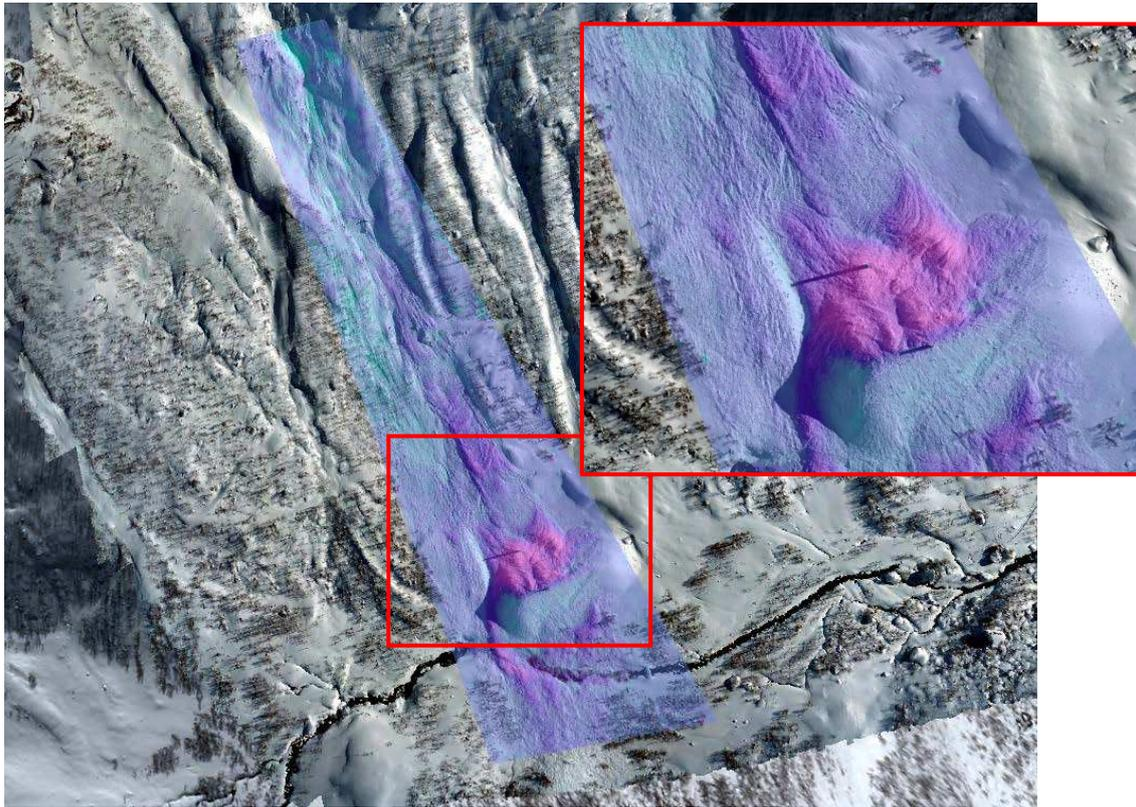
*Figure 2. Difference of UAS-derived surface models generated before and after the avalanche experiment (warmer colours indicate snow accumulation, while cooler colours represent snow erosion); difference map displayed on top of UAS-derived orthomosaic and high-resolution satellite image.*
